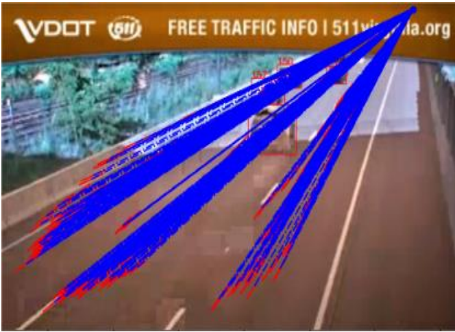
Fig. 2. RANSAC algorithm used on vehicle paths to estimation VP1. VP1 represented with the intersection of blue lines
